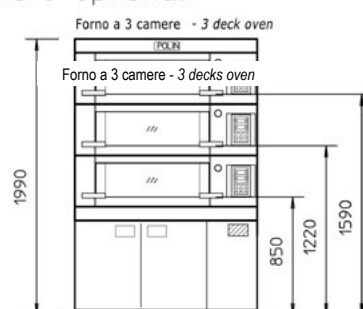
Forno con cella o basamento carenato (ruote optional) Oven with proper or base-box (castors optional)
